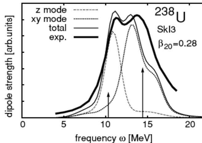
FIG. 7. Dipole strength in the prolate ground state of  $^{238}\text{U}$  computed with SkI3. The total strength is shown as well as the strengths for the separate modes. The experimental result from [3] is shown for comparison. The estimated peak positions (see Sec. III A) are indicated by arrows.
